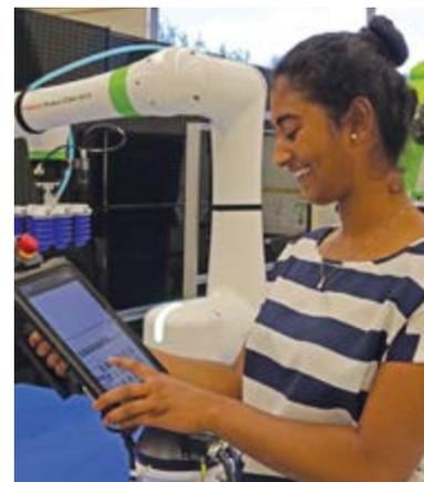
With the all new FANUC CRX Tablet Teach Pendant – simple programming becomes reality. Easily program and teach points with the CRX Tablet Teach Pendant. The drag and drop interface for lead-through teaching and simple programming is easy with no prior robotic experience needed.
