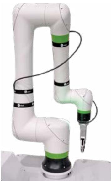
Adding to CRX Application flexibility is FANUC force sensors. A force sensor gives the robot the sense of touch and feel. This is very useful for [material removal, including sanding, buffing, and deburring, as well as assembly applications](#). Force sensors are plug and play with FANUC's cobots including the CRX.
